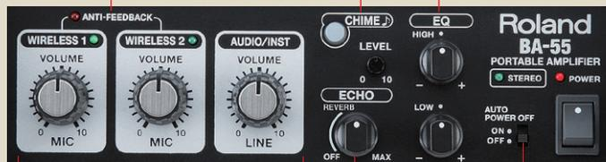
■ 3-channel mixer function for instant, hands-on control of the line input and two mic inputs.
